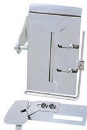
P044A zwijacz do gurtu. WAISTBAND MACHINE WAISTBAND LINING ATTACHMENT
